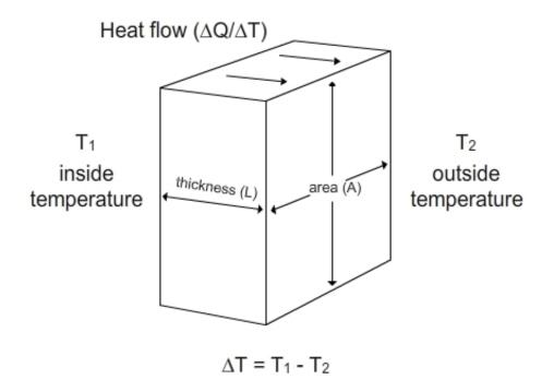
Factors that affect heat conduction through a solid material.
