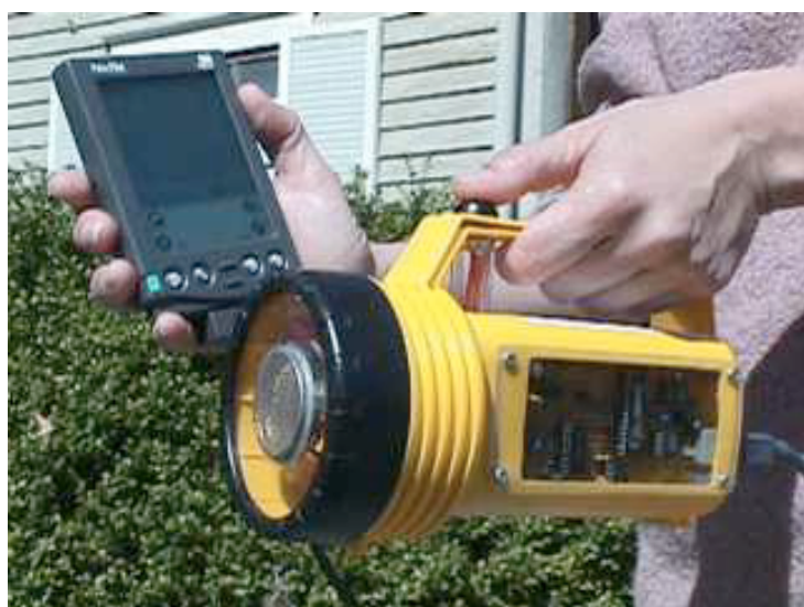
Figure 3. The smart motion detector interfaced to a Palm handheld computer. The
