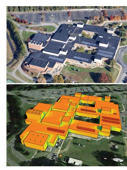
**Figure 2.** Upper image: The 3D model of a school in Google Maps. Lower image: Energy3D's shading visualization shows the distribution of solar radiation on the roof.
