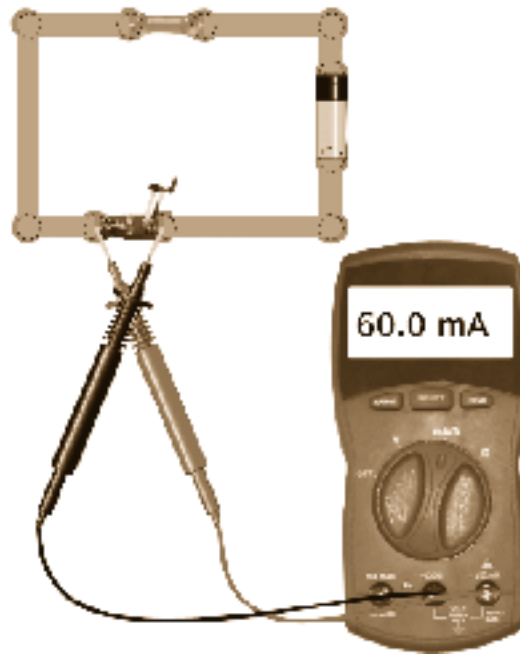
Figure 1. Simulated circuit and multimeter set up to measure the current through the resistor.
