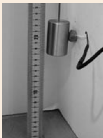
Figure 4. In “Heating by Hitting,” students measure the energy (as heat) after a weight collides with a lump of clay.
