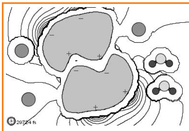
Figure 1. Smart surfaces. This is a model of molecular recognition between polymers. Each bead represents an amino acid. By changing the properties of amino acids, students can alter the effectiveness of the recognition.
