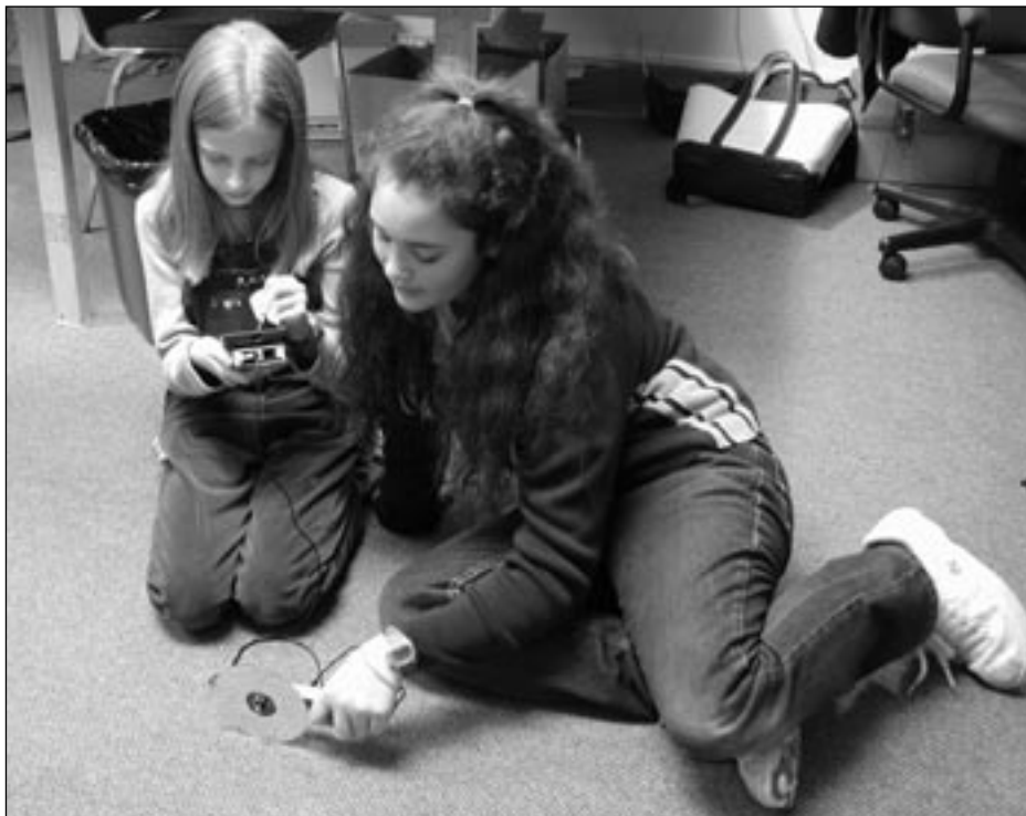
The CCSmartWheel probe, attached to a Palm handheld computer, uses an optical encoder on a CD-ROM wheel to record motion. The wheel can be easily attached to a cart, meter stick, or pulley, making it very versatile.
