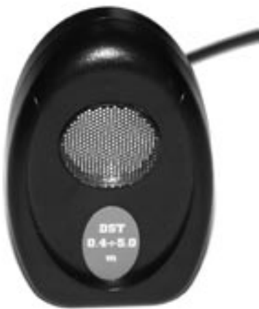
Figure 6. The ImagiWorks Sonar Ranger attaches to a Palm handheld computer. It allows a student to experiment with the concept that motion can be measured and represented on a graph.
