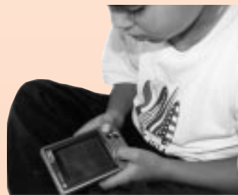
Casio's Cassiopeia handheld is not wireless yet, but they have a compact flash expansion slot normally used for memory expansion that they say by sometime this fall could be used for wireless Ethernet expansion.
