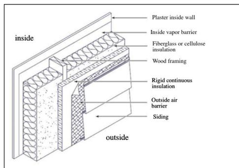
Air spaces inside walls may or may not provide some insulating value. If they are wider than about 2 cm, convection loops form and heat is easily transferred across them. If they are narrower than that, convective loops do not form and they provide insulating value.
