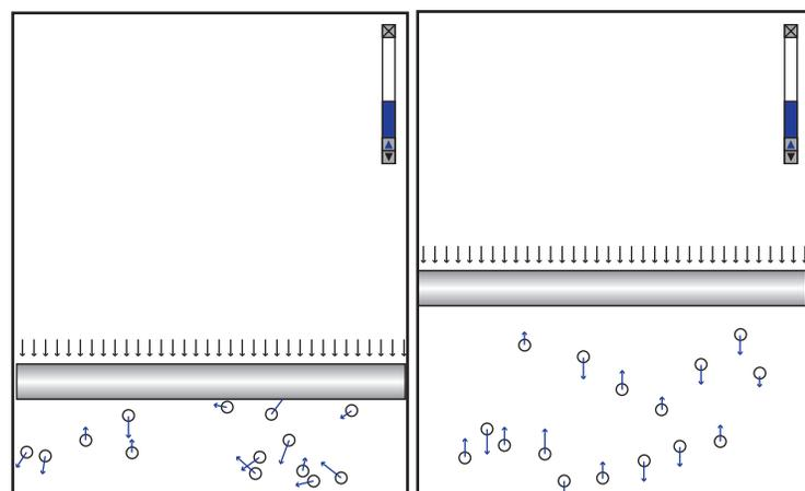
**Figure 3. A simulation created by a student showing that if all particles move only perpendicular to the piston, the volume of the gas will be twice as much as if they are moving in all directions, if the external pressure, temperature, and number of particles are identical.**
