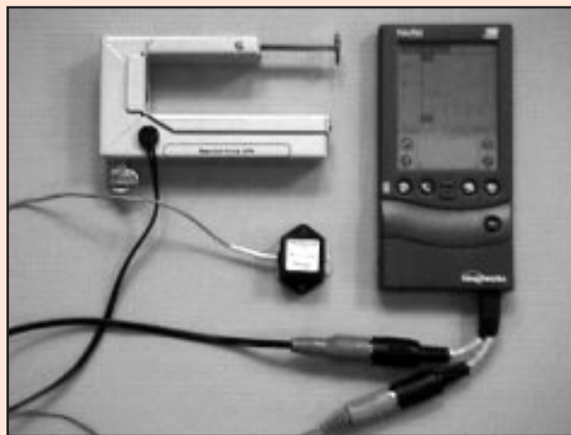
Figure 1. Palm computer with an ImagiWorks interface and Vernier probes.
