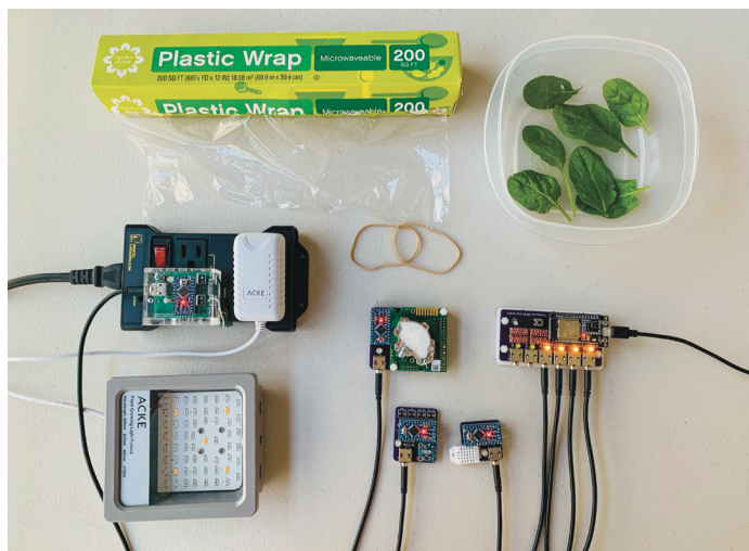
Figure 1. A Dataflow hardware kit including (from top left): plastic wrap, a container of spinach leaves, a custom-built “IoT” sensor hub, carbon dioxide, light, and temperature/humidity sensors, an LED grow light, and an IoT relay.
