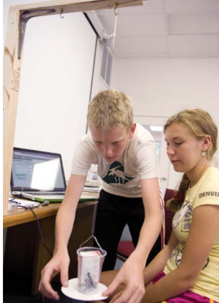
Figure 1. A distance sensor measured the up-and-down motion of various masses hung from various springs.
