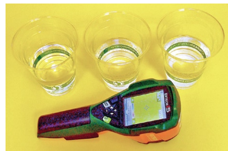
Figure 1. Pure water, salt solution, and baking soda solution in three cups, alongside a Flir I5 IR camera.
