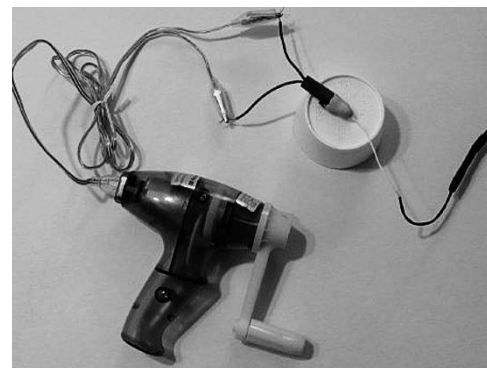
Figure 2. Generator connected to light, with sensor embedded in clay.
